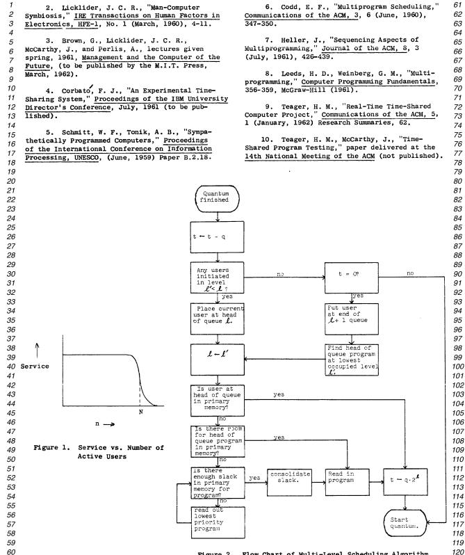
Figure 2. Flow Chart of Multi-Level Scheduling Algorithm
